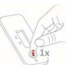
4. Holding the buffer bottle vertically, add 1 drop of buffer to the specimen well (S) of the test cassette.
